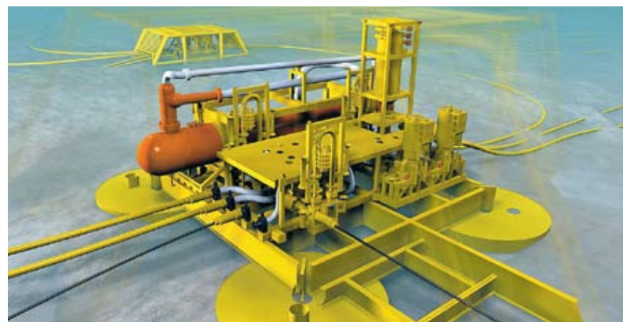
EXTRACTING WATER AND SAND: Subsea separation of water and sand from the wellstream on Tordis helps to relieve limited processing capacity on Gullfaks, and allows the first of these fields to produce more oil and gas. The water and sand are injected in a nearby formation.
