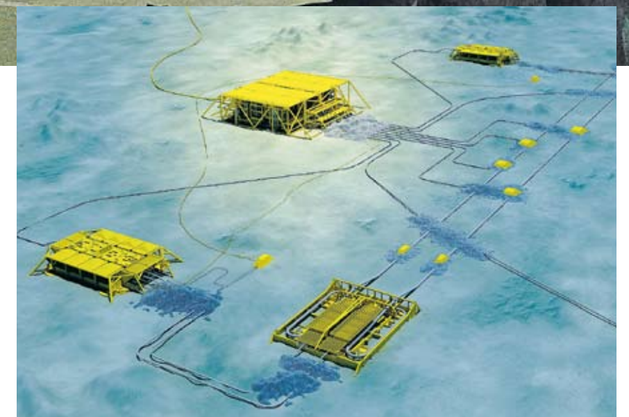
UNDER PRESSURE: A pilot plant to test subsea gas compression is to be installed on Ormen Lange in the Norwegian Sea. This could eliminate the need to build a new platform and help to boost profitability.
